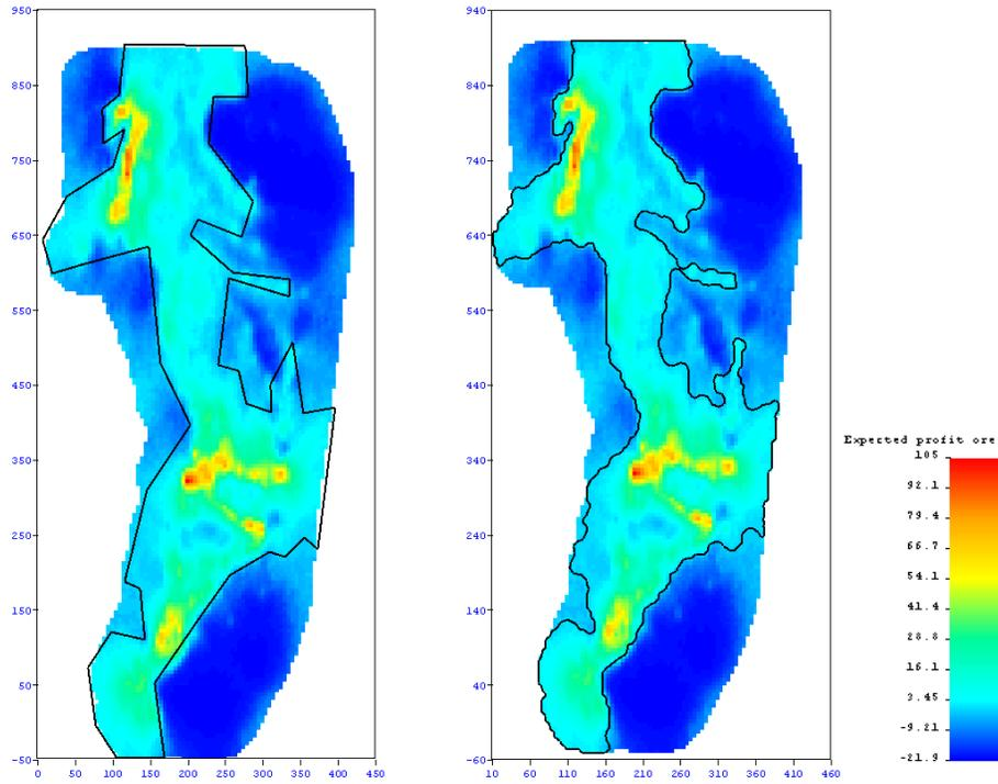
**Figure 5:** Expected profit model with initial and final dig limits.
