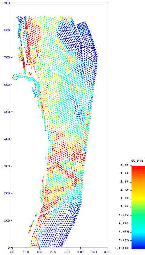
**Figure 3:** Blasthole locations on copper porphyry bench.
