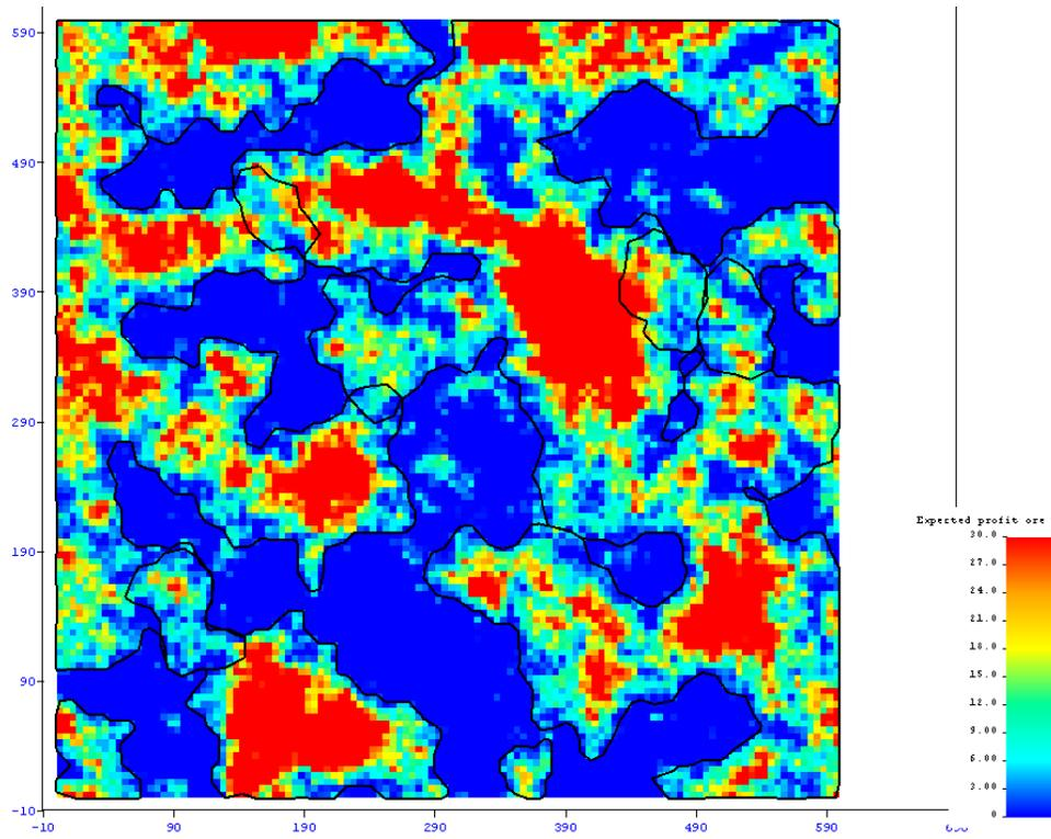
**Figure 8:** Profit model with optimized dig limits.
